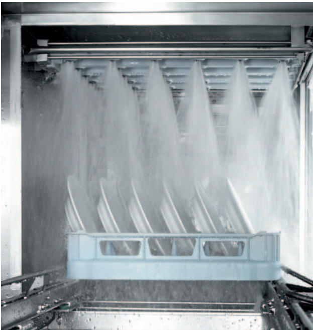
Without continuous rack conveyor motion: Contact with the rinse water is not uniform*
