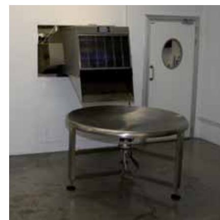
Outlet for discharging bags onto rotary table
